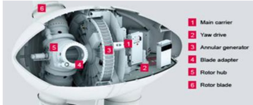
Figure 2 - Gearless wind turbine [ 3]
