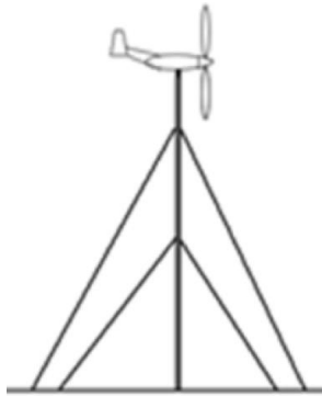
Figure[11]: Guyed Mast
